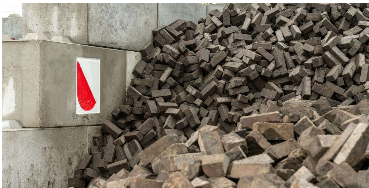
Prefabricated stackable concrete blocks for the storage of pavers at Trechterweide. City of Utrecht, 2025. © City of Utrecht
